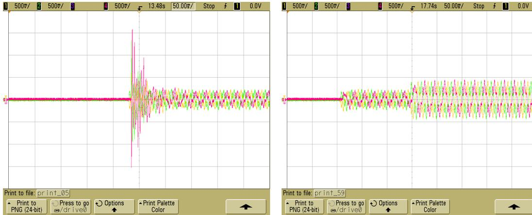
the flow when tuning / detuning capacitor bank is put into random use
